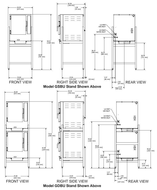
Note: Dimensions do not change for variations in Model Numbers. Bullet Feet and Flanged feet have a 1" adjustment.
